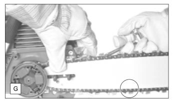
Turn the chain tightener (C/6) to the right (clockwise) until the chain engages the guide groove of the bottom side of the bar (see circle). Press the guide bar against the housing with your left hand.
